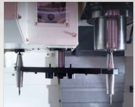
■ Auto Tool Change (T-T) 1.8 sec. ■ Auto Tool Change (T-T) 4.2 sec.< NXV1680B >
